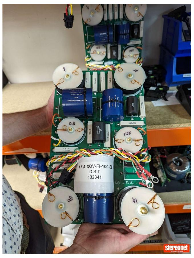
The active crossovers are fourth-order Linkwitz-Riley designs with additional all-pass filters at the two crossover points, httconnected directly to the drive units at line level. The result of this method should be more accurate handling of the crossover points and improved control, thanks to the direct connection between the power amplifier and the drive unit.
